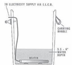
The heater operates within a temperature range approximately 22 to 32 degrees C. The temperature to which the heater is pre-set should suit the needs of the feeder. The neon light within the heater lights up when the heater is functioning and will light intermittently when the operating temperature is reached. The thermometer provided with the feeder may be used to check the water temperature.
